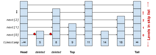
Figure 5: Concurrent Skip List (CSL) used for tiers 1 & 2 of 3tSkipMT
